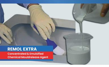
First dilute REMOL EXTRA concentrate in the proportion of 1:6 with water, using a clean container and stirring thoroughly until evenly mixed. and demolding or stripping Apply the REMOL EXTRA 1:6 water dilution to the face of the formwork by spray, brush or cloth. Only one coat should be applied.
