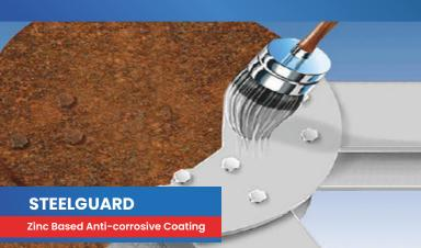
The first coat should be applied to all areas by the use of suitable brushes or rollers to achieve a uniform coating with wet film thickness not less than 175 microns. The second coat of STEELGUARD should be applied exactly as detailed above, again achieving a wet film thickness not less than 175 microns.
