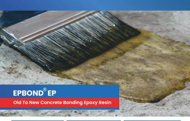
The entire contents of the 'hardener' tin should then be poured into the 'base' tin and the two materials thoroughly mixed using a suitable slow-speed drill and mixing paddle for 2 minutes until a fully uniform colour is obtained then apply using brush.
